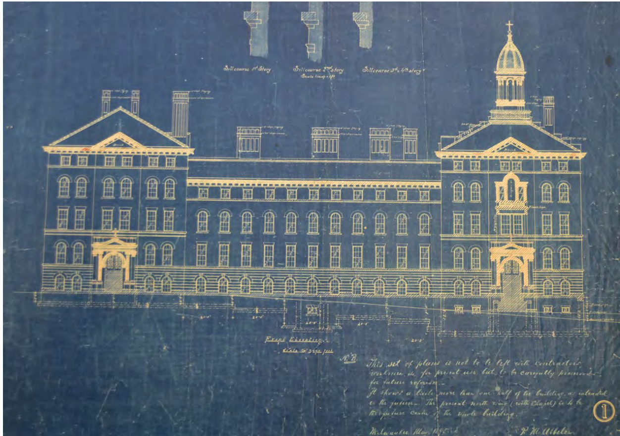
Figure 12. The east elevation, as originally designed in 1895 with the Chapel wing at the north end. The note at the bottom right explains the intention that a north wing would be constructed in future to allow the Chapel wing to be the center of the building. Schnetzky & Liebert, 1895. Plans held in the SSND Archives.
