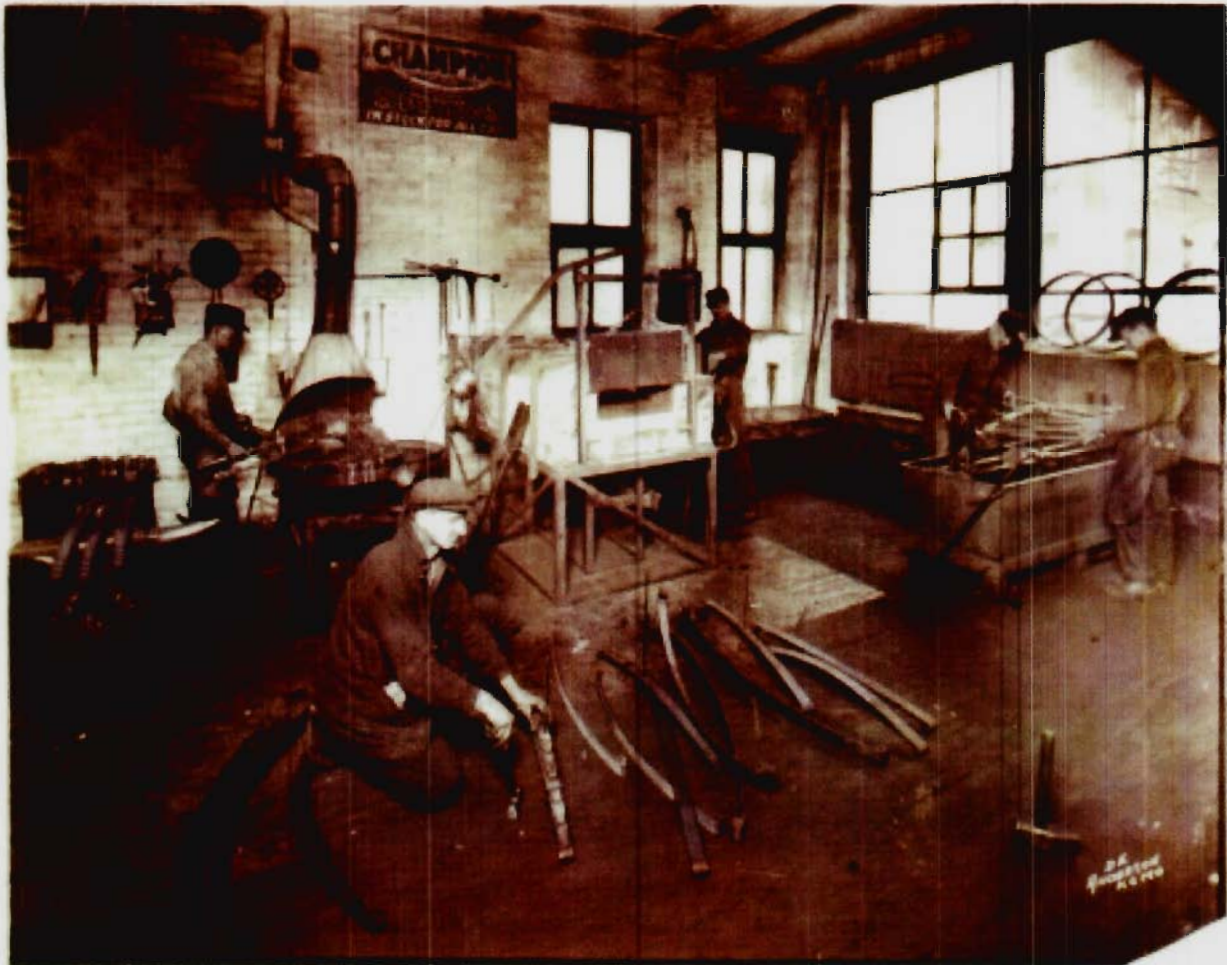
Interior of Hesse Carriage Company repair shop Repair crew working on new auto springs Courtesy: Group Hesse archives.
